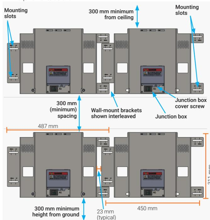
(Dimensions shown are for the 450 mm wall-mount bracket. See the image below for the 600 mm bracket.)
