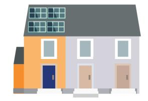
In this scenario, a housing association finances a PV system for a tenanted dwelling as part of its portfolio to improve the energy efficiency of its housing stock. The property is an end terrace home located in London built to Future Homes Standard levels and is fitted with a 2.5kWp PV system; and an 8kW battery.
