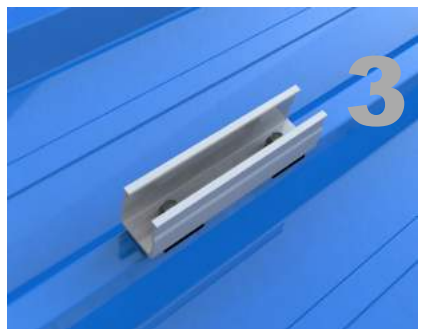
Fasten the mini rails with metal sheet roof with 2pcs of rubber pads and 2pcs st6.3*25 tapping screw.
